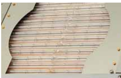
Quartz heater lamps array, adapted in size to the wafer to be processed. Several quartz lamps are regularly spaced within a cooling system.
